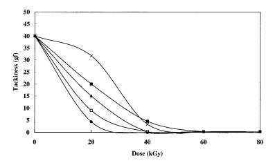
**Figure 3** Effect of irradiation on the tackiness of RVNRL film coated with 80% HEMA/20% *n*-BA: (- $\times$ -) control; (- $\blacktriangle$ -) 5% sulfuric acid; (- $\bullet$ -) wet film dipping; (- $\blacksquare$ -) 4% aluminum sulfate; (- $\Box$ -) 0.5% aluminum sulfate (mix).
