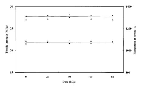
**Figure 6** Tensile strength (Ts) and elongation at break (Eb) of coated and uncoated RVNRL film at various irradiation doses: (- $\Delta$ -) uncoated (Ts); (- $\bullet$ -) uncoated (Eb); (- $\Delta$ -) 80% HEMA/20% *n*-BA (Ts); (- $\bigcirc$ -) 80% HEMA/20% *n*-BA (Eb).
