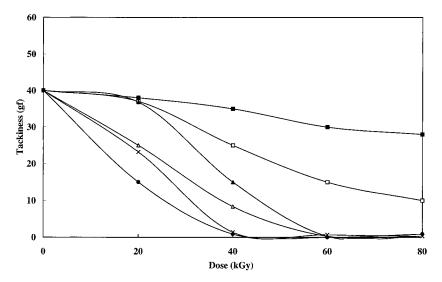
**Figure 2** Effect of irradiation on the tackiness of RVNRL film coated with various monomer mixtures: (- $\blacksquare$ -) 20% HEMA/80% *n*-BA; (- $\Box$ -) 20% AAc/80% *n*-BA; (- $\blacktriangle$ -) 50% HEMA/50% *n*-BA; (- $\triangle$ -) 80% HEMA/20% *n*-BA; (- $\times$ -) 50% AAc/50% *n*-BA; (- $\bullet$ -) 80% AAc/20% *n*-BA.
