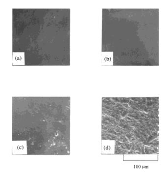
**Figure 7** Scanning electron micrograph of hydrogelcoated RVNRL film: (a) uncoated RVNRL film (control); (b) uncoated RVNRL film (irradiated at 80 kGy); (c) coated RVNRL film with 80% HEMA/20% *n*-BA (irradiated at 20 kGy); (d) coated RVNRL film with 80% HEMA/20% *n*-BA (irradiated at 80 kGy).
