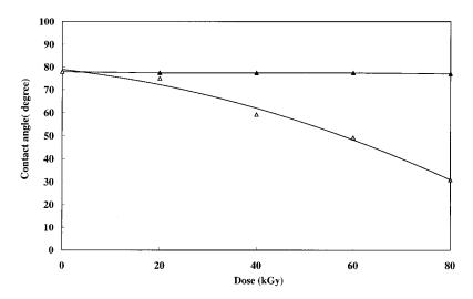
**Figure 4** Effect of irradiation on contact angle of coated and uncoated film:  $(-\Delta)$  uncoated;  $(-\Delta)$  80% HEMA/20% *n*-BA.
