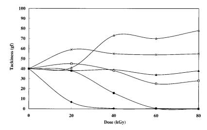
**Figure 1** Effect of irradiation on the tackiness of RVNRL film coated with various monomers:  $(-\triangle)$  *n*-BA;  $(-\times)$  NVP;  $(-\triangle)$  uncoated;  $(-\Box)$  DMAEA;  $(-\blacksquare)$  HEMA;  $(-\bullet)$  AAc.
