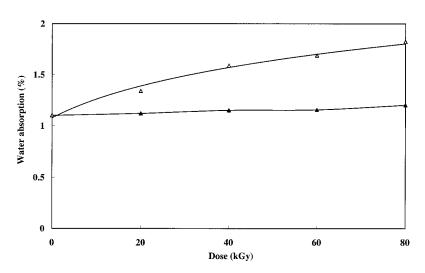
**Figure 5** Water absorption of coated and uncoated RVNRL film at various irradiation doses:  $(-\Delta -)$  uncoated;  $(-\Delta -)$  80% HEMA/20% *n*-BA.
